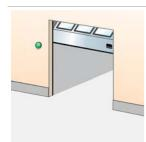
One or two green warning lights indicating the open position of the door by continuous light signal.
