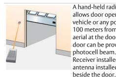
A hand-held radio transmitter allows door operation from a vehicle or any position within 50-100 meters from the receiver and aerial at the door. For closing, the door can be provided with a photocell beam.
