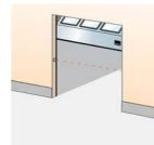
A set of a photocell transmitter and receiver is installed in the door opening. If the photocell beam is interrupted during closing, the door will stop in less than 30mm and reverse to the fully open position.
