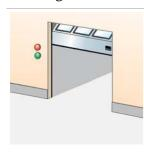
If traffic through a door needs to be directed; two red and two green traffic lights can be installed to indicate traffic direction. From the side where a vehicle is first detected to approach the door, the green traffic light comes on. The opposing side shows a red traffic light. Traffic from this direction must give way to the other. Usually installed in e.g. parking garages. Installed on the inside and outside wall beside the door.
