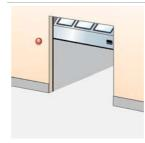
Two red warning lights giving information on the current door behaviour. Flashing light before or during door movement. Optional: Continuous light before and during door movement. Installed on the inside and outside wall beside the door.
