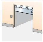
An extra control box is installed outside the building or inside close to the door if the main control unit needs to be installed away from the door opening. Installed on the inside or outside wall beside the door.
