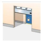
Developed for climate control or safety; If door A is open, door B cannot be opened. If door B is open, door A cannot be opened. An interlocked door can remember an up-command, if selected via a micro switch.
