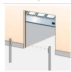
A set of photocells on pillars, on each side of the door. When a person or vehicle passes between the photocells, the beam is interrupted and the door opens. Photocells installed on pillars, away from the door.
