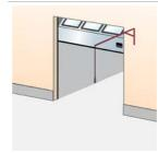
A pull-rope switch above the door opening can be operated from e.g. a forklift truck. Pulling the rope opens a closed door or closes an opened door.
