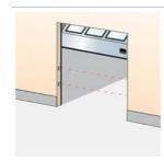
Two sets of photocell transmitter and receiver are installed in the door opening. If one or both photocell beams are interrupted during closing, the door will stop in less than 30mm and reverse to the fully open position. Installed in the door opening.
