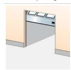
When it is unnecessary or undesirable to fully open a door, an additional switch can be used to open the door to a preprogrammed reduced opening position.
