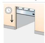
A programmable timer that closes the door after a specified time, counted from either the fully open position and/or from passing through the photocell beam. Adjustable micro switches in control unit.
