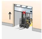
As a standard, all doors that have the impulse-close function or any form of automated closing, are equipped with a safety edge. The pneumatic sensor in the bottom seal detects any obstruction under a closing door and reverses the door.
